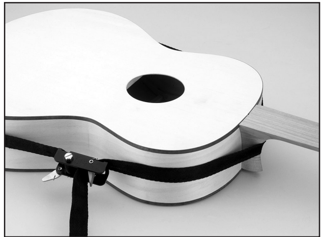
Figure 4. Clamped neck/body assembly.
